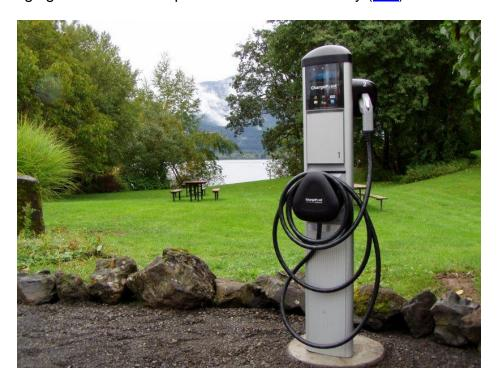
If not, you can arrange to have level 2 charging station installed at your home. According to the DOE, "the price of Level 2 residential EVSE varies, but typically ranges from \$500 to \$2,000 before installation and state or utility incentives. Typical charging time for a Level 2 EV charger is around **8 and 10 hours** from near empty to full while the average standard Level 1 EV charger will take up to 20 hours to fully charge."
