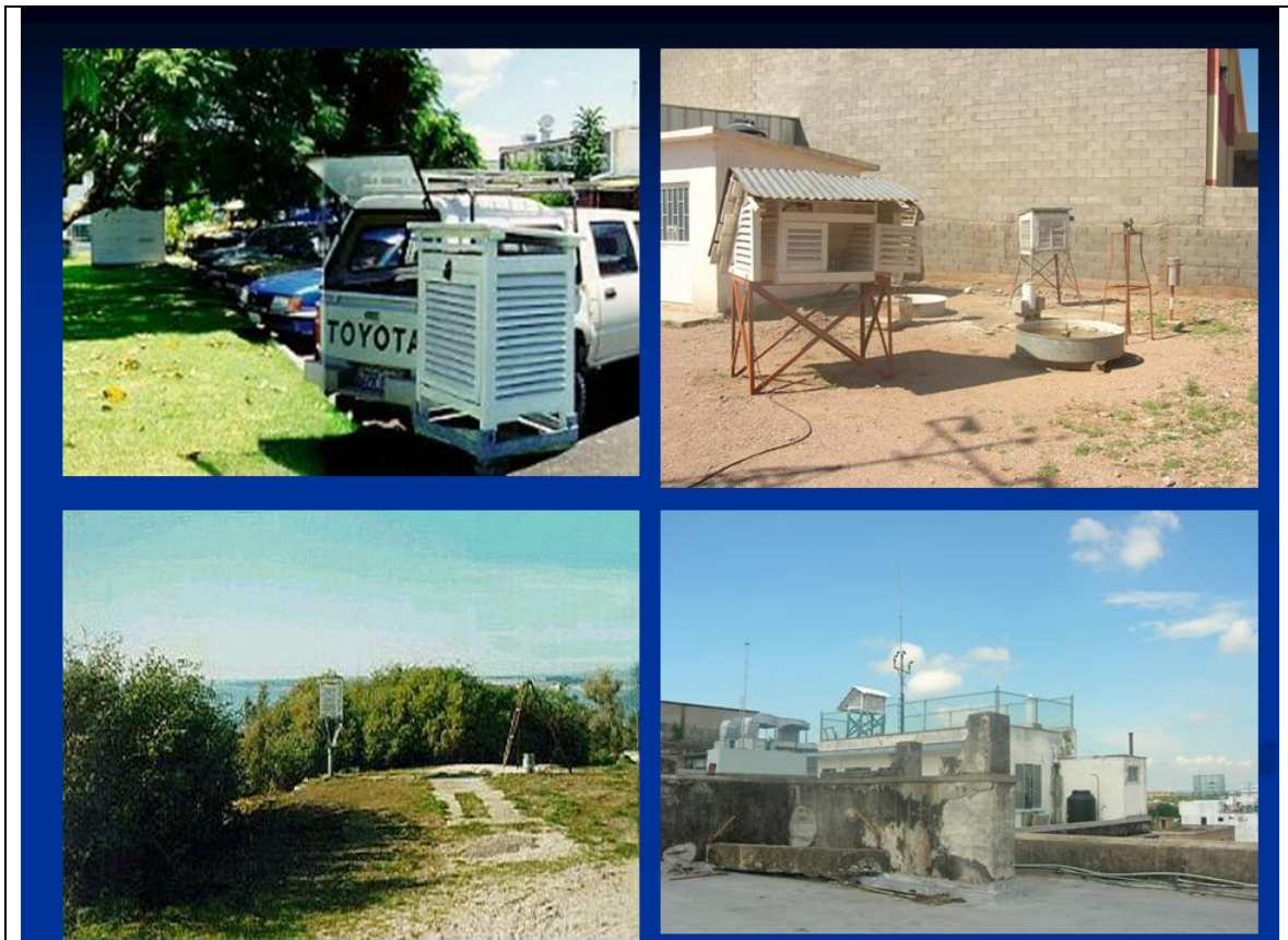
Examples of shelters whose siting does not meet WMO standards. Land use changes such as building construction, paving parking lots right up to the shelter, increase in height of vegetation blocking the proper ventilation needed, or placing the shelter on the roof of a building. Each of these lead to a warm bias. (photos from John Daly and Roger Peilke Sr)
